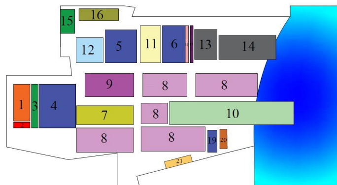
Fig. 6. Current layout ((1) Steel Plate and Profile Stockyard, (2) Profile Cutting Area, (3) CNC Cutting Area, (4) Pre-Assembly Area – 1, (5) Pre-Assembly Area – 2, (6) Pre-Assembly Area – 3, (7) Panel Production Area, (8) Block Production Area, (9) Block Buffer
