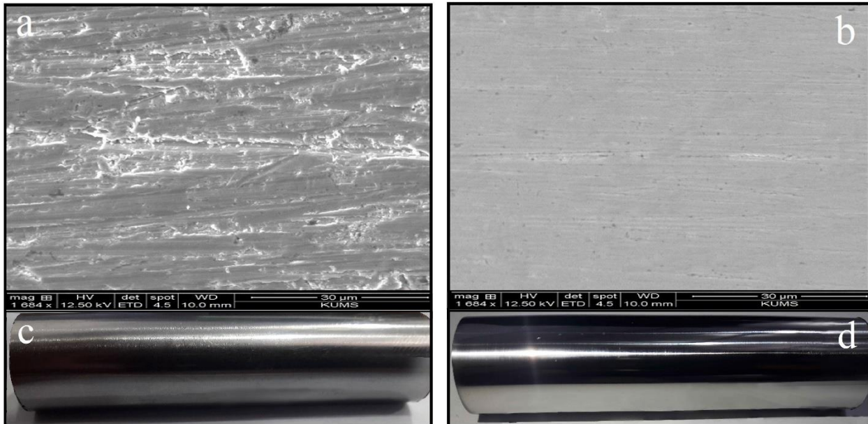
Fig. 12 SEM images and surfaces of workpiece; (a and c) before, and (b and d) after process.
