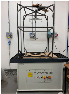
(a) Omnidirectional pendulum energy harvester mounted on a shaker table
