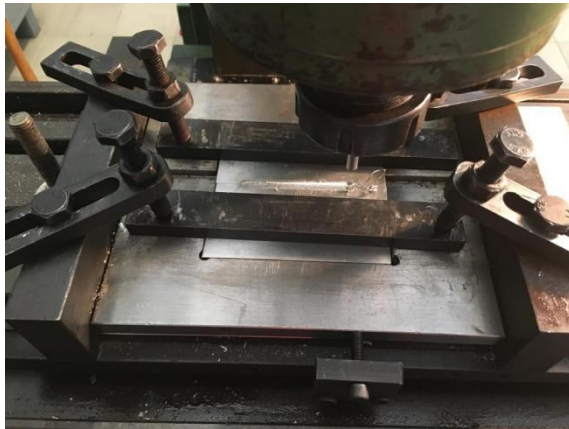
(a) (b) Figure 1. (a) Welding setup of 0.5mm thick plate (b) tool design
