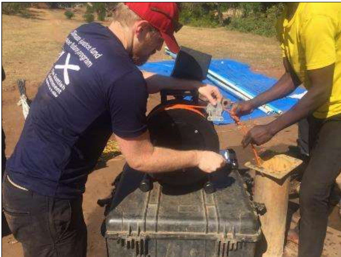
Figure 43a. Deploying the Envirotech EI-150 camera downhole as part of the borehole forensics analysis of Chimkamda Borehole
