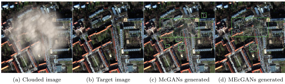
Figure 4. Example of Berlin dataset test image results with \eta_{\text{NIR}} = 1\% . for the generated images (c)-(d), the differences w.r.t. the target image (b) are highlighted by the contours (white) and their bounding boxes (green).
