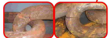
Mooring chain crack failure due to fatigue [4]
