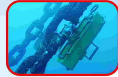
Indirect load measurement Inclinometers installed on top chain. Courtesy: pulse
