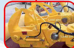
Load pin measurement Mooring line termination at the hull of Statoil's (now Equinor) Hywind spar floater. Load monitoring pins mounted on mooring quick release hooks from Mampae
