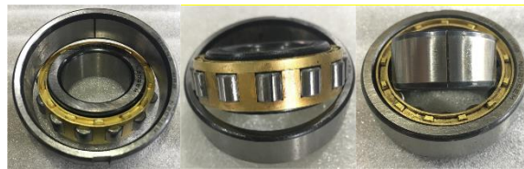
Fig.17. Three failure bearings used in QPZZ-II bearing fault test rig.
