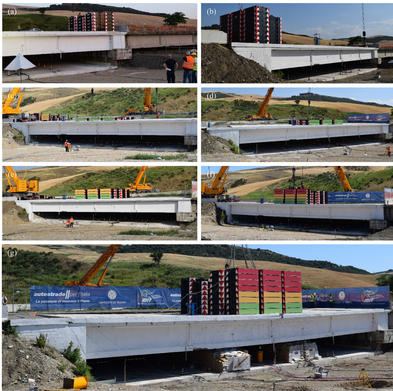
Fig. 10 Pictures of the Alveo Vecchio viaduct during the loading phases: a PP–4800 kN; b PA–4800 kN; c P1–1200 kN, d P2–2400 kN, e P3–4800 kN, f P4–7200 kN, and g P5–9600 kN
