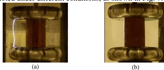
Fig. 7. Open shutter photographs showing post-breakdown channel location for: a) a smooth (machined) Ultem surface, and b) a knurled Ultem surface.
