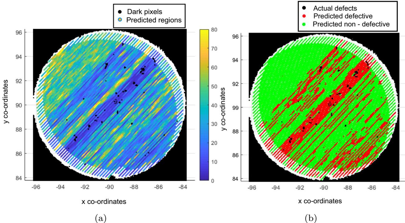
**Fig. 2** **a**  $\bar{e}_p(t)$  calculated along the hatch lines of layer 42. The defective regions of the corresponding CT image, with a gray scale value less than 80, are shown in black. **b**  $\bar{e}_p(t)$  less than 20 are indicated in red, whilst  $\bar{e}_p(t)$  higher than 20 are indicated in green
