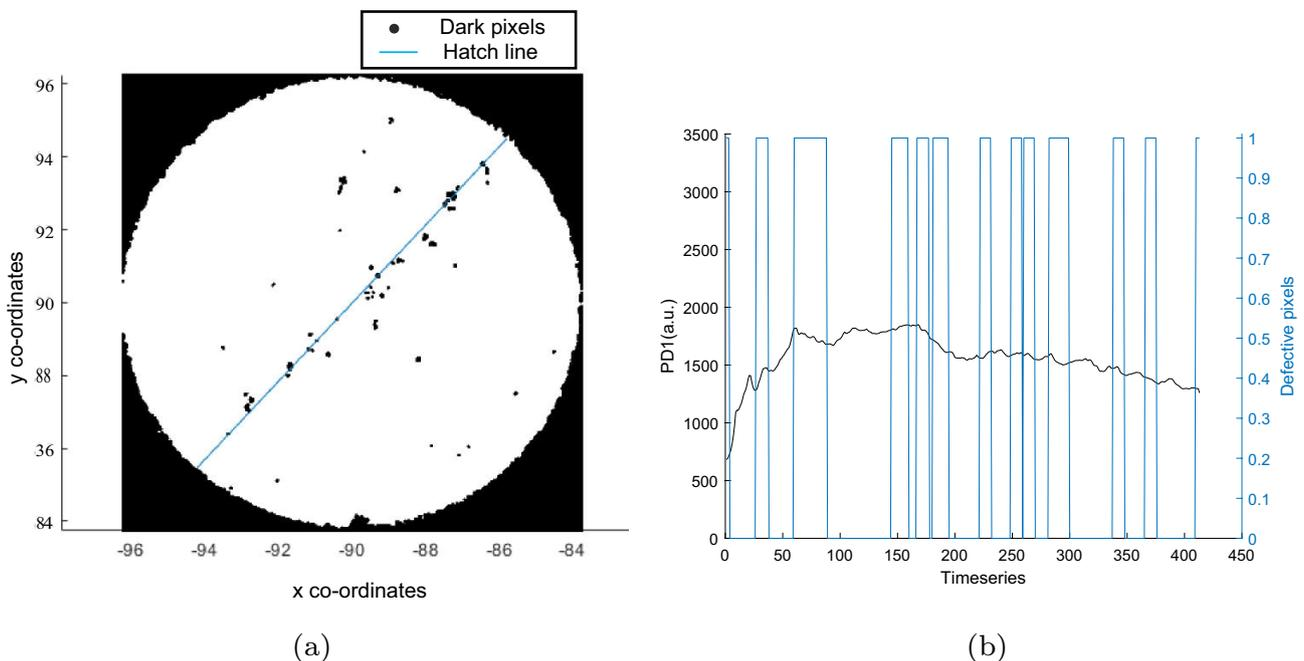
**Fig. 1** **a** A hatch line which passes through defective regions with dark pixel values (grayscale < 80) identified on a CT image. **b** Corresponding photodiode signal behaviour where blue line indicates, 1–defective and 0–non-defective
