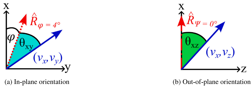
Fig. A.1. Definition of (a) in-plane, \theta_{xy} , and (b) out-of-plane, \theta_{xz} , fibre deflections in a two dimensional Cartesian coordinate system. A unit vector, \hat{R} , represents a prescribe angle in each orientation while \varphi = 4^\circ in the xy -plane and \psi = 0^\circ in the xz -plane. The \theta_{xy} and \theta_{xz} are determined as the difference between the prescribed angles ( \varphi or \psi ) and the fibre orientation vector, \vec{v} = (v_x, v_y, v_z) , from the structure tensor analysis.
