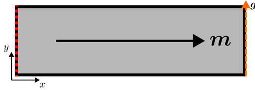
FIGURE 1. Experiments of Section 5.2: View from above of the FeCoSiB bar of dimensions (20\ell_{\text{ex}}, 6\ell_{\text{ex}}, 6\ell_{\text{ex}}) .
