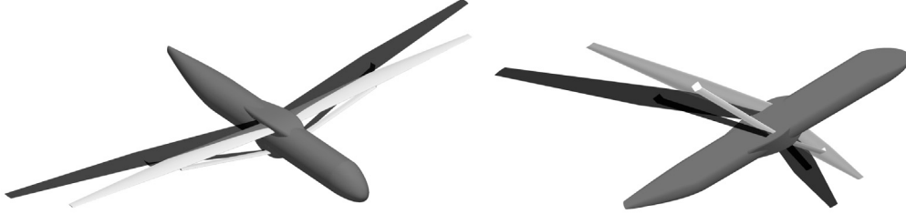
Fig. 2. Overlay of the SBW configuration at the minimum (white) and maximum (black) bounds of the geometrical parameter space.
