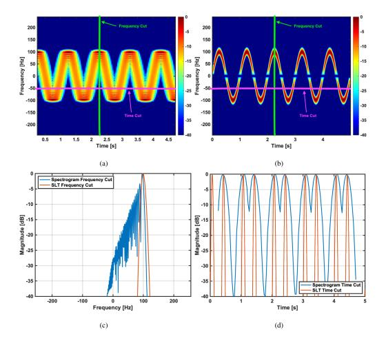
Fig. 1: a) Spectrogram of the simulated signal x(t), b) its SLT, c) cut in frequency, d) cut in time.
