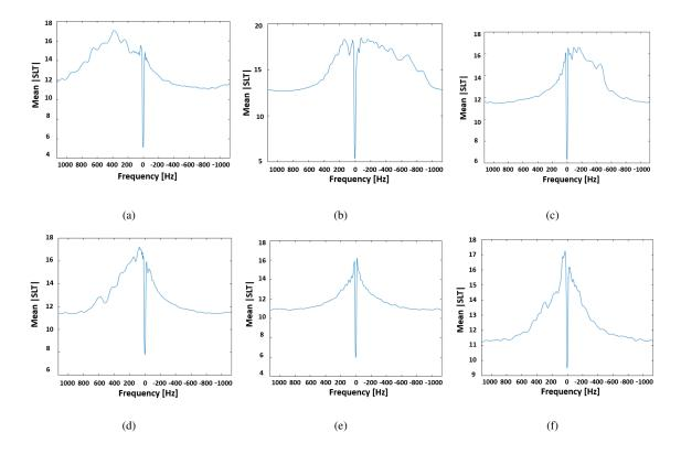
Fig. 5: *MFP of SLTs respectively for a) walking approaching the sensor, b) receding the sensor, c) sitting, d)* standing up, e) drinking, f) picking up an object.
