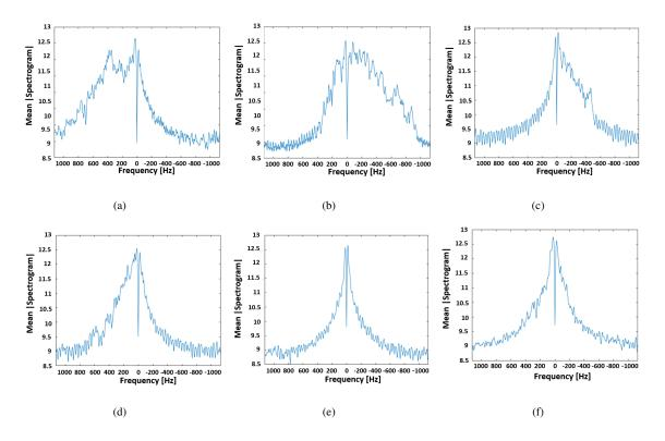
Fig. 4: *MFP of spectrograms respectively for a) walking approaching the sensor, b) receding the sensor, c) sitting, d) standing up, e) drinking, f) picking up an object.*
