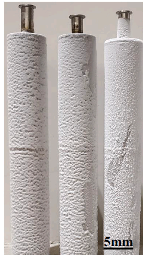
Fig. 6. Cryogenics shock test effect on Cu-SS joints.
