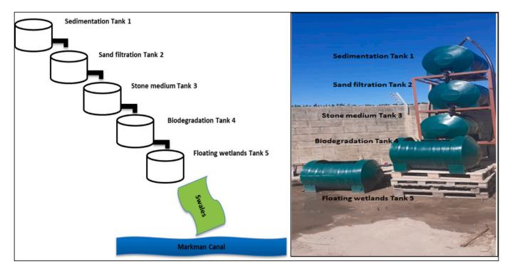
Fig. 2. Schematic diagram and photograph of the SuDS treatment train.
