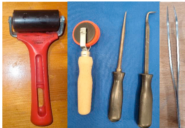
Figure 3 - Reworking tools, left to right: hard compaction roller, soft compaction roller, straight pick, L-shaped pick, tweezers.
