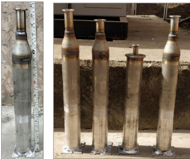
Fig. 6 Samples are prepared for vacuum and thermal shock test
