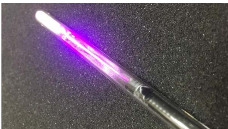
Figure 11. Fibre-optic 'pig-tail' traceably calibrated phosphor thermometer. Excitation (blue light) yields phosphor emission (red light), giving a purple appearance.
