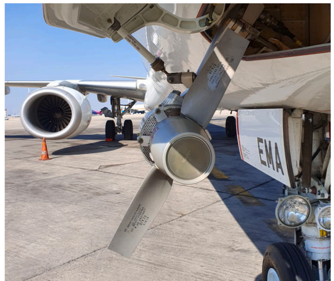
Fig. 2. The Ram Air Turbine (RAT) on modern aircraft (SASHAX41, 2019).
