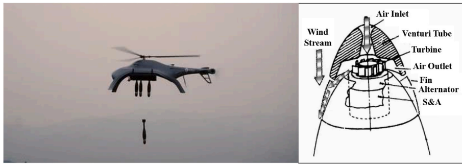
Fig. 3. The mortar shell with energy harvesting turbine (Andersen, 2017; CCTV, 2019).
