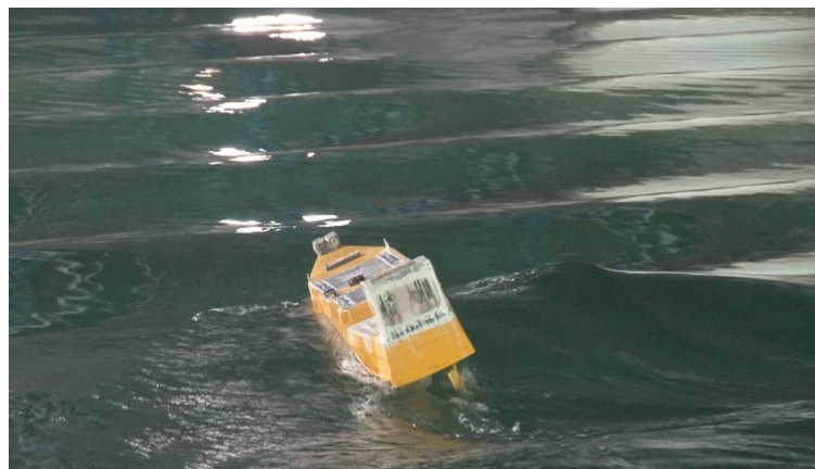
Figure 2. The free-running experiment of loss of stability in CSSRC.
