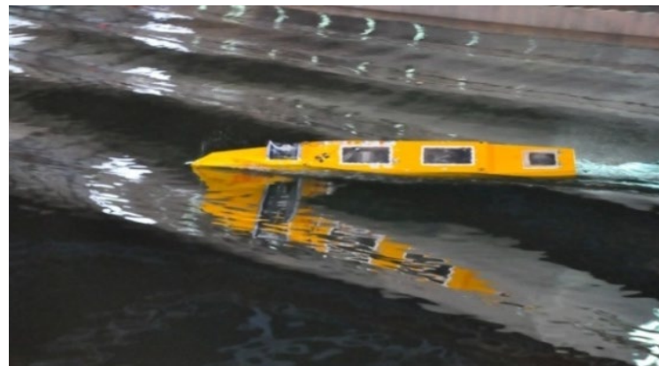
Figure 1. The free-running experiment of broaching in CSSRC.
