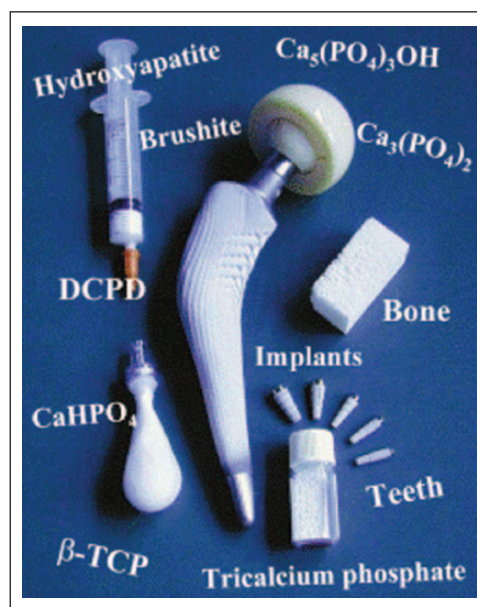
Figure 6. Examples of biomedical applications of CaP based materials (e.g. \beta -tricalcium phosphate, dicalcium phosphate, dicalcium phosphate dehydrate, tricalcium phosphate and calcium apatite) used in form of coating for hip prostheses and dental screws, porous bone graft, bone cements and pastes. Adapted with permission from Dorozhkin et al. 159
