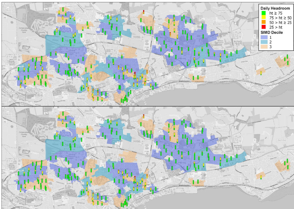
Fig. 14. Comparison of the generalised approach (top) and the localised (bottom) in more deprived areas (SIMD deciles 1, 2 and 3) at 100% penetration.
