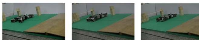
Deformation to Forward H configuration and Forward creep through the arched door
