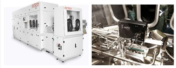
Figure 8. (a) AIXTRON G4 MOVPE Planetary Tool (courtesy of AIXTRON SE). (b) EpiCurve *in-situ* monitoring tool (courtesy of LayTec AG).
