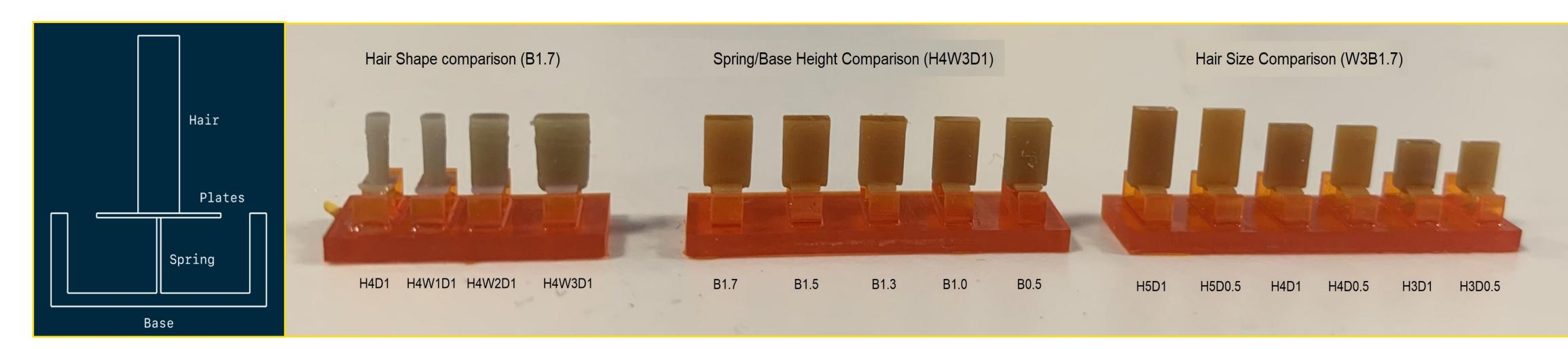
The sensors are printed by using an Asiga MAX X27 3D printer. The displacement of the hair was then measured using a 3D-Laser Doppler Vibrometer (Polytec MSA-100) and a speaker. The conducted tests changed the hair shape and size or the base/
