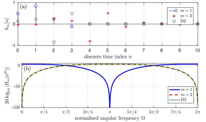
Fig. 3. Paraunitary matrix completion with (a) impulse responses and (b) magnitude responses of the two extracted filters; for comparison, D2 marks the highpass filter of the Daubechies-2 filter bank.
