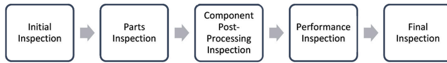
Fig. 2. An overview of the key stages within remanufacturing inspection activities as found in the case study primary research.
