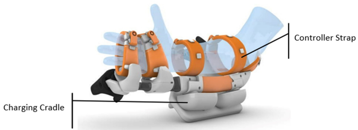
Figure 7. The bespoke VR controller developed in PRIME-VR2.
