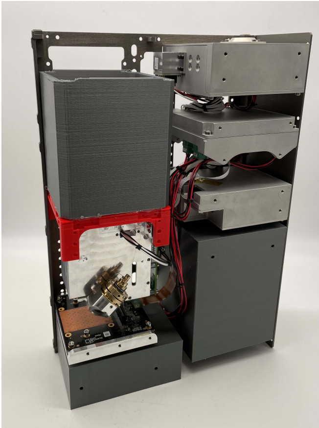
FIG. 24: All the Prepared Modules Inside the 6U CubeSat Structure
