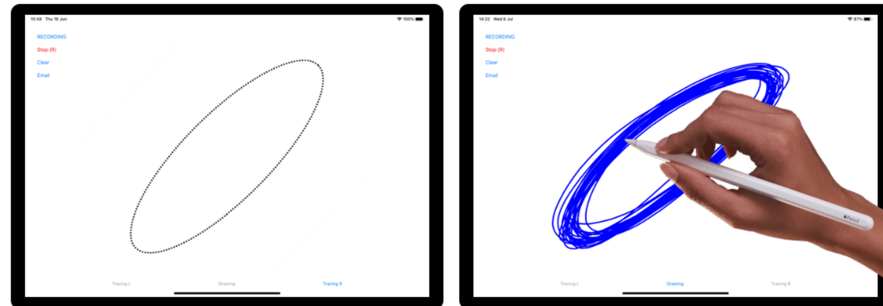
Figure 1. Participants used an Apple Pencil to first trace an elliptical trajectory on an iPad Pro 11-inch tablet and then draw ellipses on an empty canvas. Timestamped trajectories and force during tracing and drawing activities were recorded.
