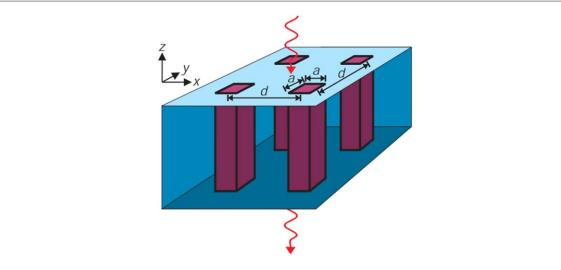
**Figure 5.** The model system:  $a \times a$  square hole made on a  $d \times d$  grid is divided into the surface of an ideal conductor. From [208]. Reprinted with permission from AAAS.
