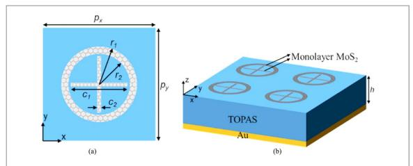
**Figure 6.** Presented absorber with MRC layer. (a) Top view. The geometric parameters:  $p_x = p_y = 60 \ \mu\text{m}$ ,  $r_1 = 20 \ \mu\text{m}$ ,  $r_2 = 16 \ \mu\text{m}$ ,  $c_2 = 2 \ \mu\text{m}$ ,  $c_1 = 30 \ \mu\text{m}$ . (b) The structure of the MRC array and the bottom gold layer are divided by a thin TOPAS dielectric layer with a thickness,  $h = 26 \ \mu\text{m}$ . Reprinted from [243], Copyright (2021), with permission from Elsevier.
