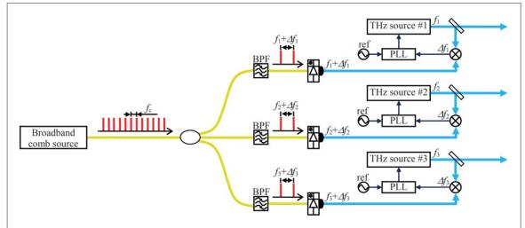
**Figure 4.** Schematic diagram of concept of locked phase multifrequency terahertz source system. © 2016 IEEE. Reprinted, with permission, from [47].
