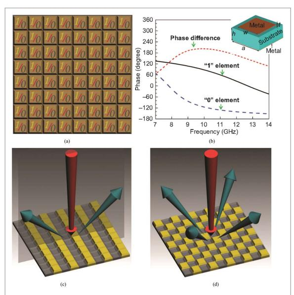
**Figure 9.** The surface of the 1-bit numeric element and the surface of the encoded element. (a) The surface of a 1-digit element consists of two kinds of parts: '0' & '1'. (b) Square metal patch cell for achieving '0' & '1' and According to phase response in the frequency field. (c, d) Two 1-bit periodic coding element surfaces, which determine beam scatter by design coding sequences of '0' & '1' parts: (c) 010101..., 010101..., and (d) 010101.... / Reproduced from [274]. CC BY 4.0.
