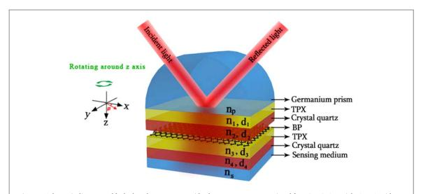
Figure 7. Schematic diagram on black phosphorus or waveguide plasmon structure. Reprinted from [245], Copyright (2021), with permission from Elsevier.
