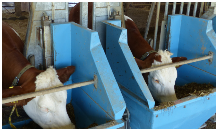
Figure 1. Hokofarm Roughage Intake Control electronic feed bin. Adapted under Fair Use from Hokofarm Group, 2021 [22].
