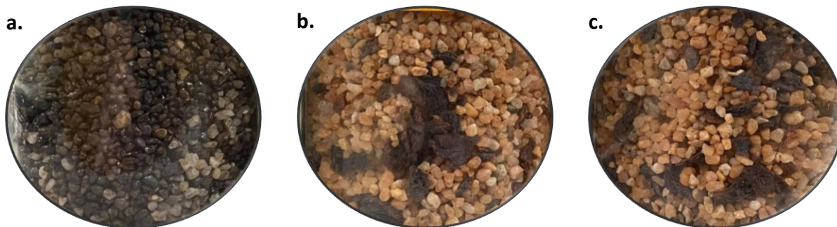
103 Figure S2-17: Experimental photos of the post-treatment ash and sand from base case I-1 from three locations within the reactor, 104 a. the top sand cap, b. the middle of the fuel bed, and c. the bottom of the fuel bed.
