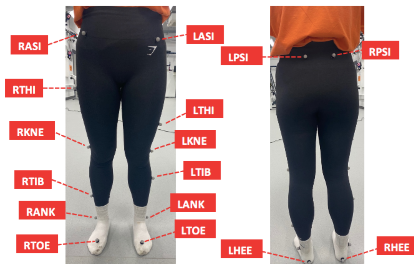
Figure 2: Marker placement using the Plug-in-Gait model.
