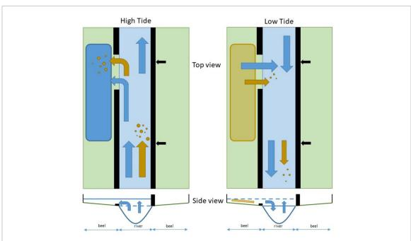
**Figure 4.** Tidal river management approach for delta landscape management showing high tide and low tide operation. Through this process of managing water flows, sediment is deposited preferentially in the floodplain, allowing agricultural improvement and increased crop production.
