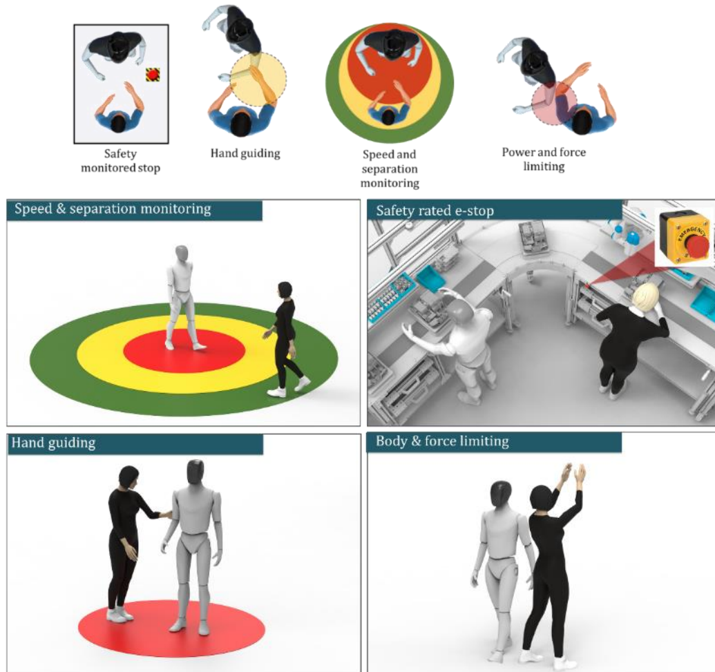
Figure 9: Illustrations of different forms of human-humanoid interaction on the manufacturing floor in the light of ISO-15066.
