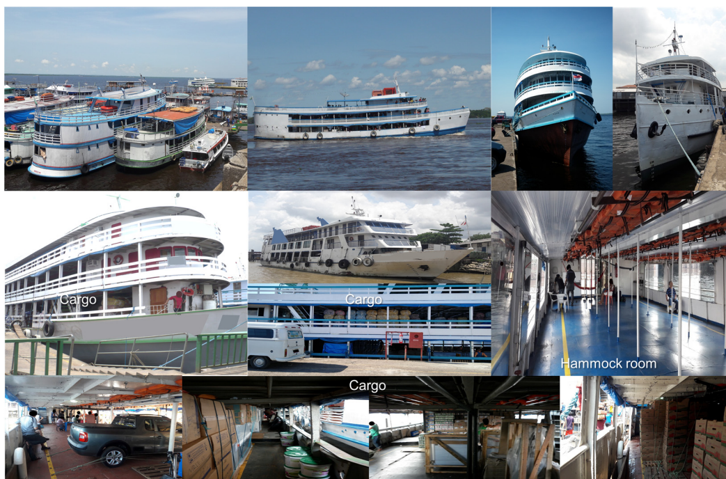
Figure 4. Long-distance vessels in the Brazilian Amazon for the transport of passengers and diverse cargo, sometimes irregularly distributed cargo. These vessels can be regionally named “gaiolas” or “recreios”. Photo credits: Ricardo de Almeida Sanches.
