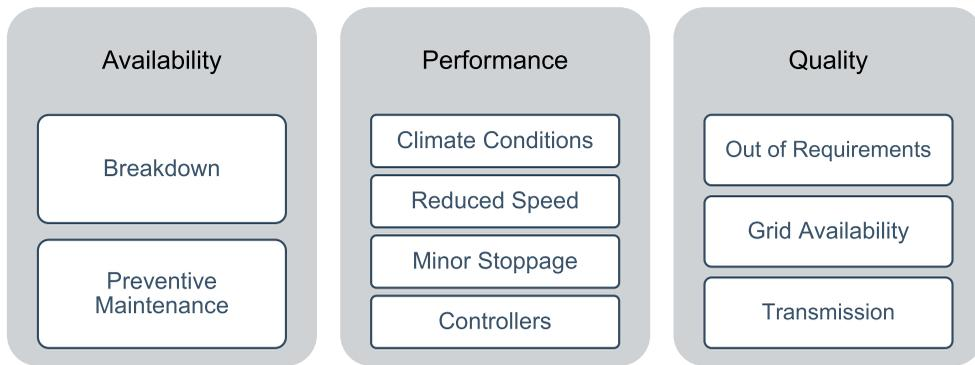
**Figure 5.** Main operational losses in wind power.
