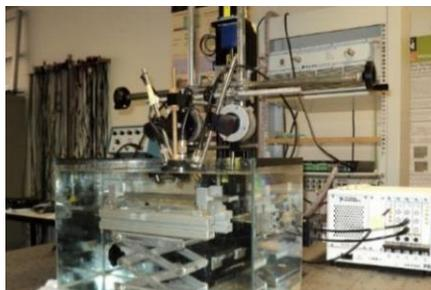
Fig. 1. Immersion ultrasonic measurement set-up.
