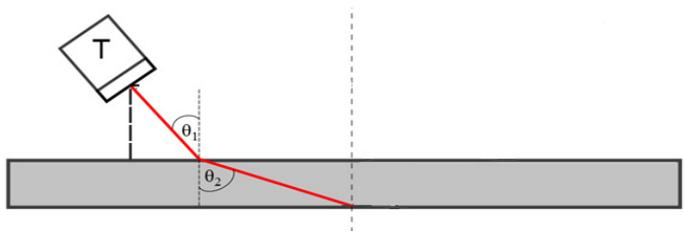
Fig. 3. Schematic representation of the ultrasonic immersion measurement set-up using a pulse echo mode for the sample analysis. The transducer/receiver is denoted by T. The vertical offset and the incidence angle remain fixed during the entire C-scan.
