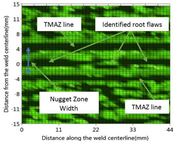
Fig. 4. Top view of the PSD analysis of oblique incident C-scan measurements for a welded 7XXX alloy sample.
