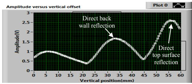
Fig. 2. Vertical scanning measurement on the weld metal to determine the ideal vertical offset to the plate and assure the acquisition of the back wall reflection.
