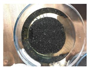
Fig. 4 Glass vessel containing the rubberised asphalt in direct contact with the water
