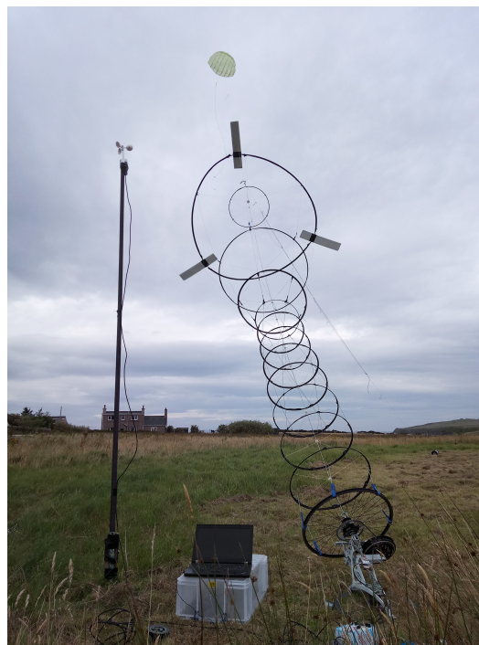
Figure 8. Image of a rigid rotor Daisy Kite prototype undergoing field tests (August 2019).
