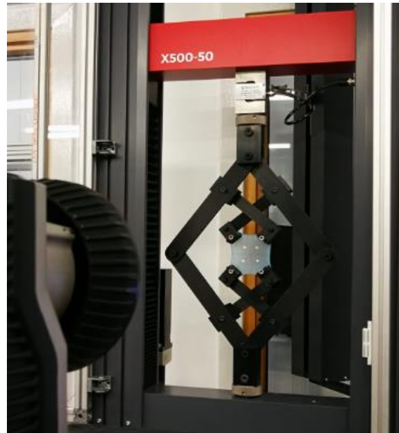
FIGURE 5: SETUP FOR BIAXIAL TESTS FOR LTR USING QUALYSIS OPTICAL MEASUREMENT SYSTEM.
