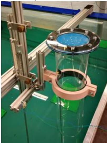
Figure 2. Dimensions of OWC and experimental setup
