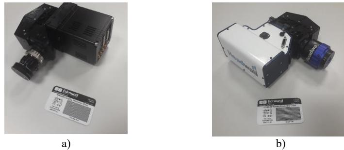
Figure 2. Hyperspectral cameras used to capture data: a) VNIR-E series (400-1000nm), and b) SWIR-640 series (900-2500nm). A resolution test chart the size of a credit card is included for scale.
