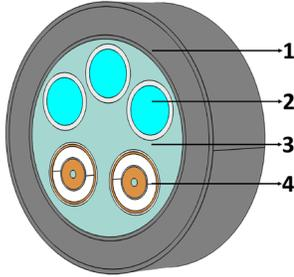
Fig. 1. The 3D structure of DC SEP. (1. the thermal insulating pipeline; 2. LNG pipeline; 3. LN<sub>2</sub>; 4. DC superconducting cable).
