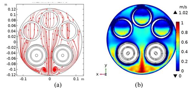
Fig. 5. The fluid field diagram: (a) the fluid velocity field streamline; (b) the fluid velocity field cloud diagram. (LNG flow rate=100L/min)
