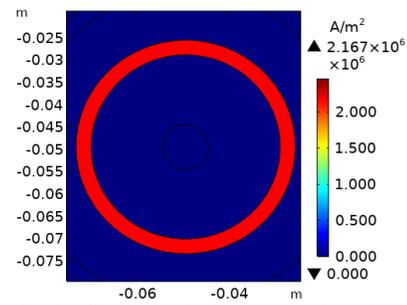
Fig. 3. Current density distribution in the cross-section of HTS cable. ( $I = \pm 1$  kA, steady state)
