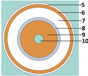
Fig. 2. The 2D cross-section of a DC superconducting cable. (5. the sheath; 6. shield layer; 7. the insulating layer; 8. the superconducting layer; 9. the copper former; 10. LN<sub>2</sub>).
