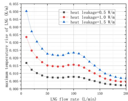
Fig. 8. The variation of the maximum temperature rise of LNG with the LNG flow rate at different heat leakage.
