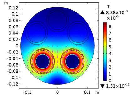
Fig. 4. Magnitude and direction of the magnetic flux density  $\mathbf{B}$  in the cross section of the DC SEP. ( $I = \pm 1$  kA, steady state)
