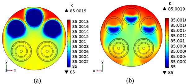
Fig. 6. The inlet and outlet temperature distribution of DC SEP: (a)the inlet; (b)the outlet. (LNG flow rate=100L/min, heat leakage=1.0W/m)
