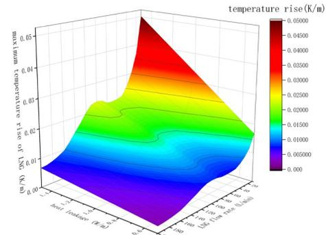
Fig. 7. The influences of heat leakage and LNG flow on LNG temperature rise.
