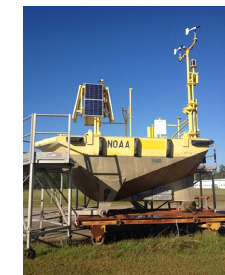
Figure 5: Photo of 6-meter NOMAD Buoy on a cradle.
