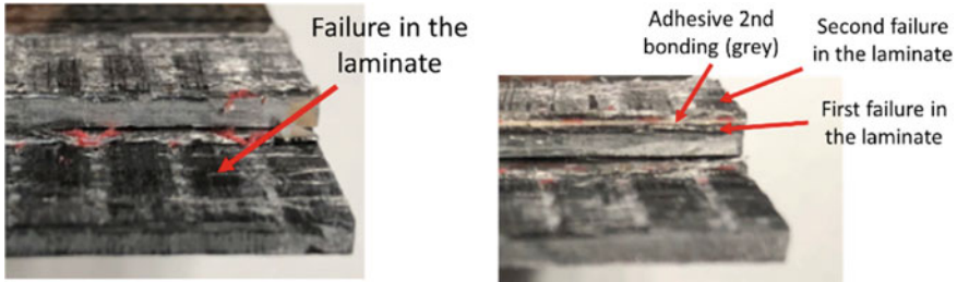
Fig. 16 Failure modes: with removing the adhesive (left) and only cleaning (right)
