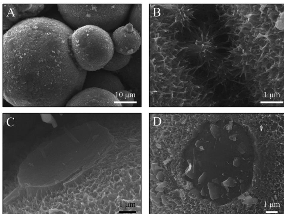
**Figure 34.** SEM micrographs showing cross growth and fracture features noted on the titanate-converted Ti6Al4V microspheres. (A,B) Cross-linking of two individual microspheres through the growth and bonding of the produced titanate nanostructures at different magnifications. (C,D) Smooth morphology of the microsphere surfaces at the failure of the bonded interface at either end of the failure. Reproduced from Wadge et al. [329], with permission from Elsevier.
