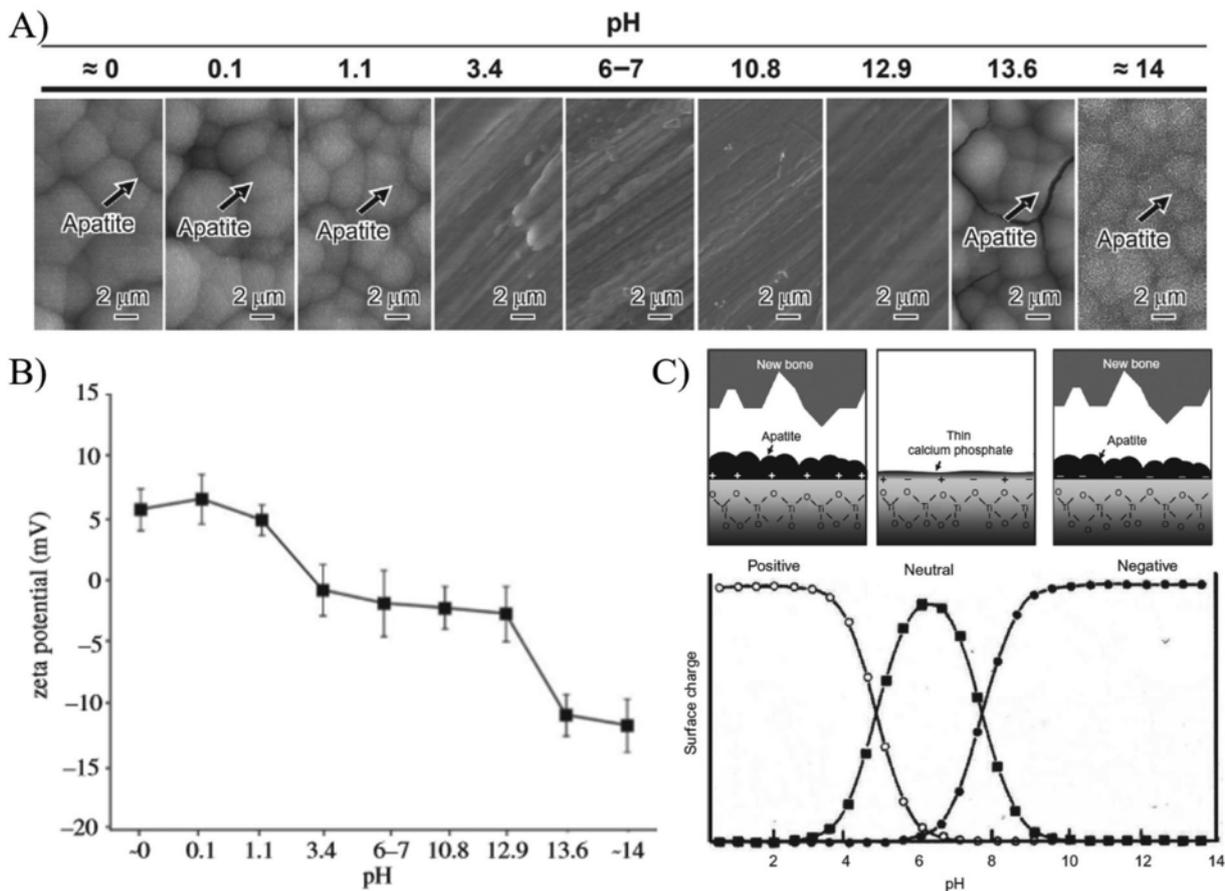
**Figure 12.** (A) Morphological changes as a function of solution pH during alkali/acid treatment of Ti substrates. (B) Zeta ( $\zeta$ ) potential measurements as a function of solution pH. (C) Representation of surface charge with respect to solution pH, and its effect on apatite formation on the surface. Figures adapted from Pattanayak et al. [154], with permission from the Royal Society.
