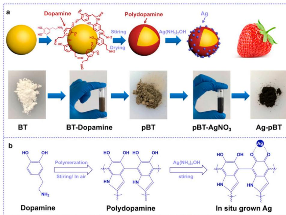
**Figure 23.** Preparation process (A) and reaction mechanism diagrams (B) of *in situ* growth of Ag nanoparticles on BaTiO<sub>3</sub>. Reprinted from Shuai et al. [258] with permission from Elsevier.
