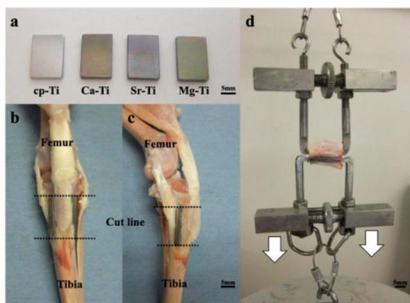
**Figure 21.** Sample appearance, implantation into the tibia, and the biomechanical test used in the *in vivo* study. (A) Cp-Ti and surface-treated Ti plates. (B,C) Representative images of the knee after sample explanation. (d) Detachment test to measure the bone-bonding strength of the implant. Reprinted from Okuzu et al. [233] with permission from Elsevier.
