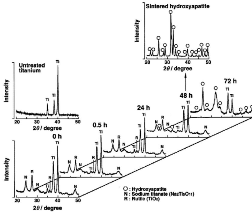
**Figure 9.** XRD spectra of sodium titanate surfaces and their transformation into apatite following submersion in SBF over 72 h. Figure reproduced from Takadama et al. [146], with permission from John Wiley and Sons.
