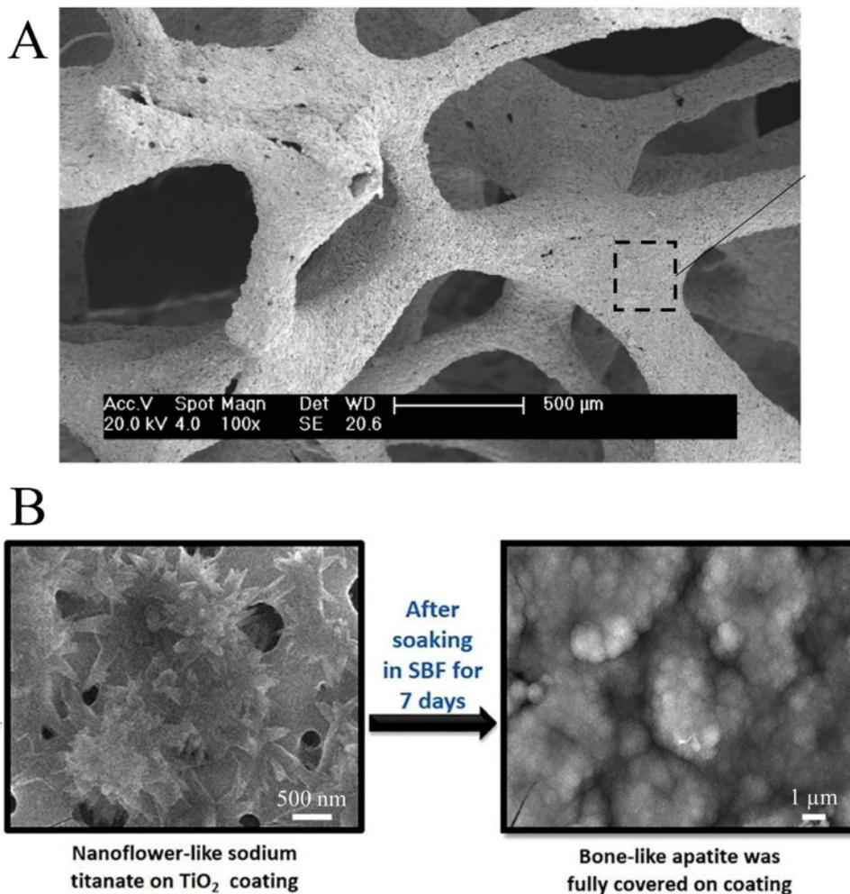
**Figure 13.** (A) SEM micrograph of hydrothermally treated porous TiNbZr scaffolds. Reprinted from Rao et al. [157] with permission from Elsevier; (B) Formation of nanoflower-like sodium titanate on a TiO<sub>2</sub> coating via anodic oxidation. Reprinted from Lee et al. [158] with permission from Elsevier.
