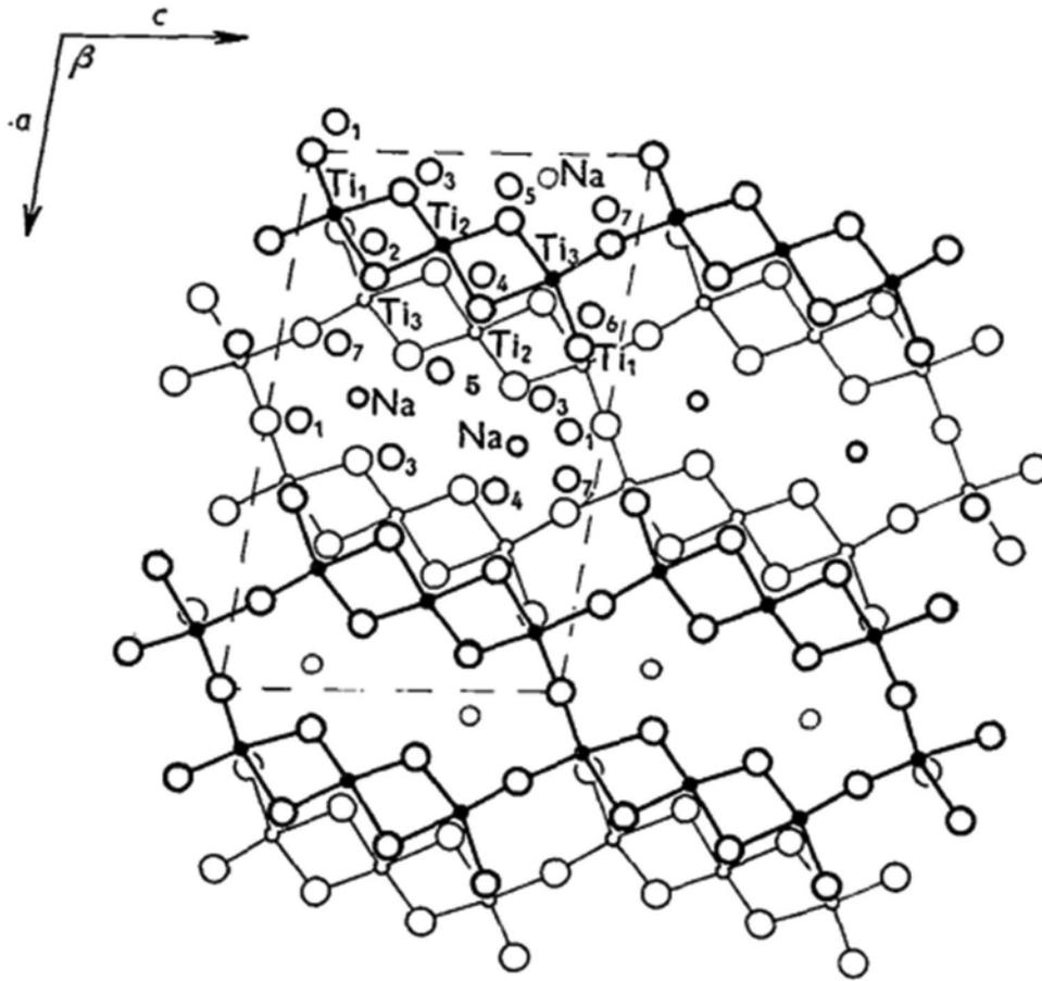
**Figure 7.** Structure of  $\text{Na}_2\text{Ti}_6\text{O}_{13}$ , as illustrated by Andersson and Wadsley [144], projected on to (010). Small circles are titanium, medium are sodium and the largest, oxygen. The atoms in heavier outline are at  $y=0$  and the lighter at  $y=1/2$ . Reproduced with permission of the International Union of Crystallography.
