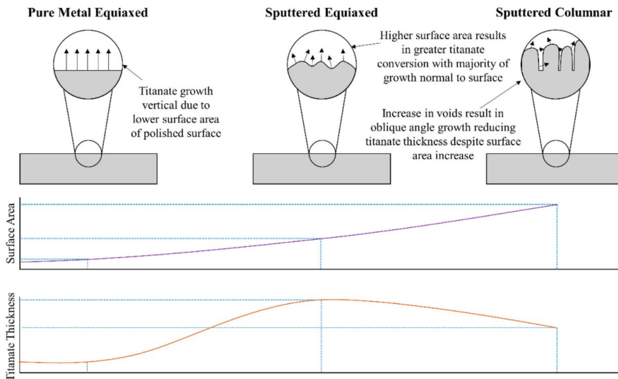
**Figure 32.** Relative correlation between the surface area of the sputtered Ti coating produced, and the relative effect on the produced titanate thickness in comparison to pure Ti metal conversion, as described by Wadge et al. [37]. The graphs at the bottom are purely a relative representation of the surface area and titanate thickness dependence.
