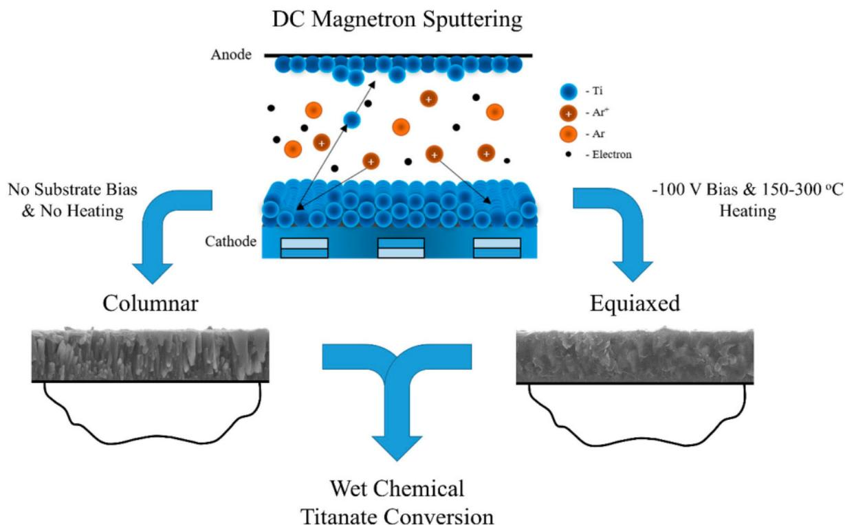
**Figure 31.** Methodology developed by Wadge et al. [37] for the wet-chemical conversion of DC magnetron sputtered Ti thin films in order to generate nanoporous titanate structures on alternative materials for biomedical applications.
