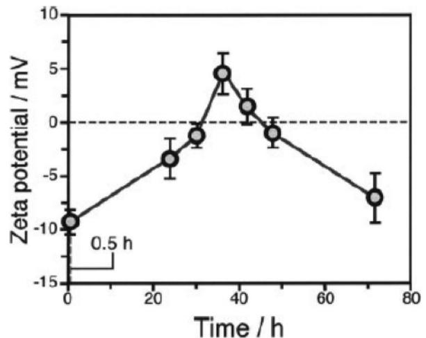
**Figure 11.** Zeta ( $\zeta$ ) surface potential as a function of soaking time in SBF. Figure reproduced from Kim et al. [147], with permission from John Wiley and Sons.
