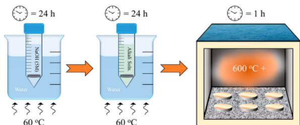
**Figure 5.** Full methodology of titanate conversion, including intermediate ion-exchange steps in order to convert the produced sodium titanate structures into alternative alkali titanates described in this review. Furthermore, the final furnace heat treatment stage is also outlined in order to increase the stability of the produced titanate structures through crystallisation.
