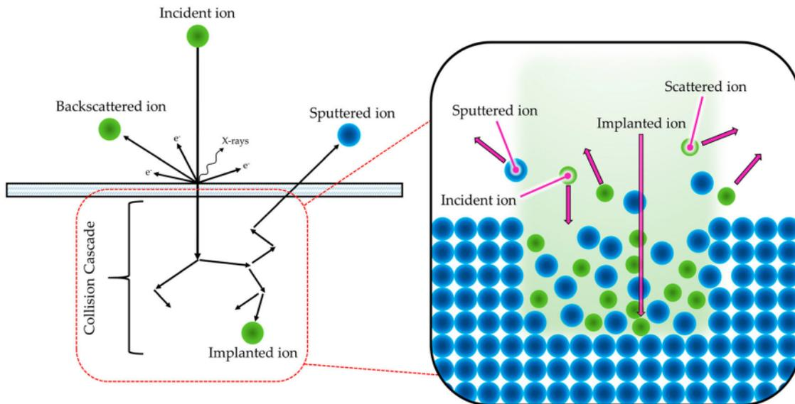
**Figure 2.** Schematic representation of ion–solid interactions, which is the principle mechanism employed for ion implantation.
