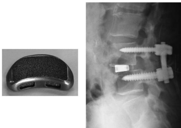
**Figure 29.** Spine fusion device of porous Ti metal subjected to NaOH, HCl and heat treatments (left-hand side) and its clinical application (right-hand side). Reproduced from Kokubo and Yamaguchi [26], with permission from Wiley.
