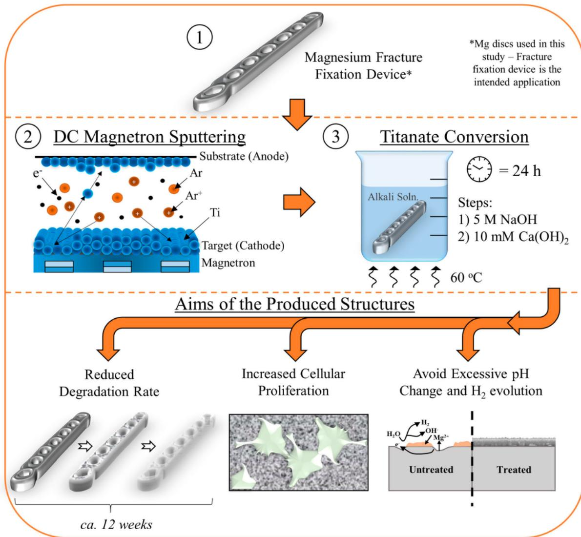
**Figure 33.** Schematic representation of the desired effect of titanate structures being applied to degradable Mg substrates, through the combination of DC magnetron sputtered Ti thin films and subsequent wet-chemical conversion [323].
