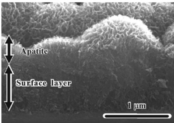
**Figure 10.** SEM image of the formation of apatite on the surface of alkali- and heat-treated titanium surfaces after 1-day immersion in SBF. Figure reproduced from Yamaguchi et al. [148], with permission from The Ceramic Society of Japan.
