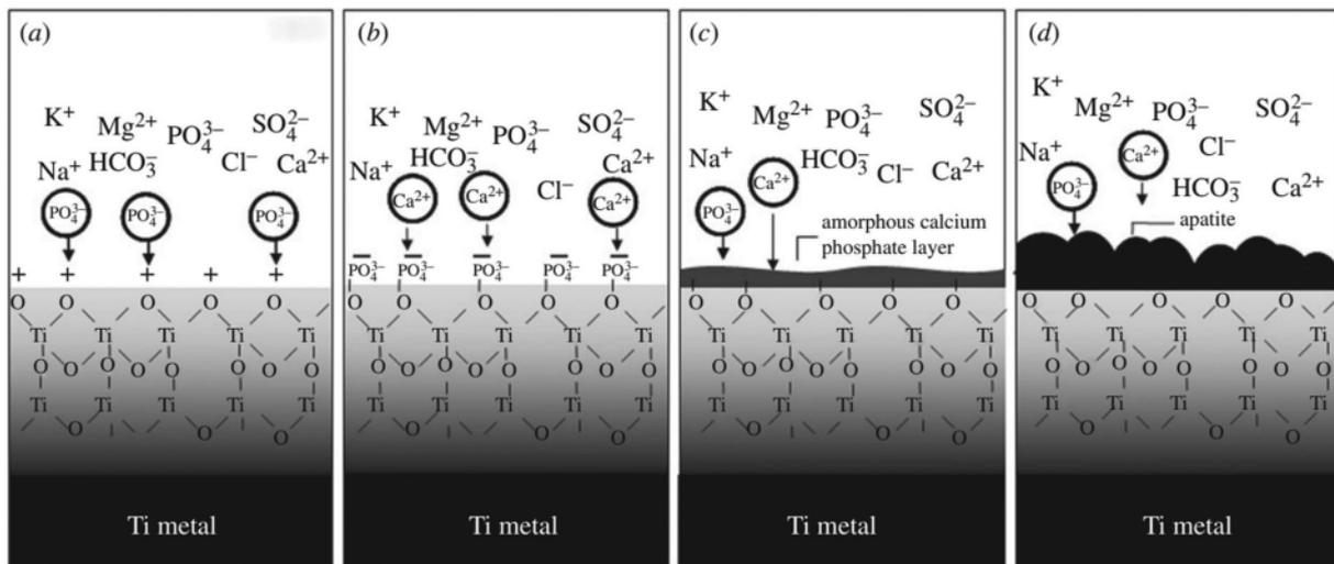
**Figure 30.** Process of formation of apatite on positively charged Ti metal in SBF. Apatite is formed by the process shown in (a–d). Reproduced from Kokubo et al. [315], with permission from the Royal Society.
