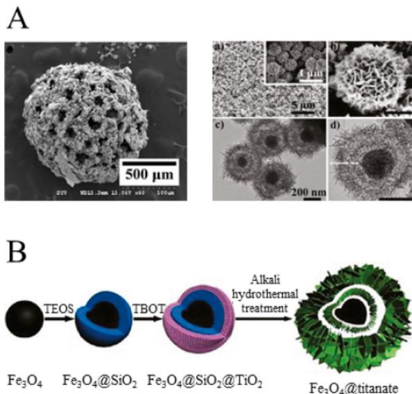
**Figure 15.** (A) SEM micrograph demonstrating the morphology of a titanium microsphere made porous through the use of a camphene porogen. Reprinted from Hsu et al. [163] with permission from Elsevier; (B) Schematic illustration of the formation process of the  $\text{Fe}_3\text{O}_4$ @titanate double-shelled yolk-shell microspheres. Reprinted with permission from Li et al. [165]. Copyright (2011) American Chemical Society.
