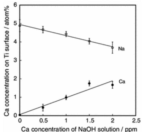
**Figure 18.** Na and Ca concentrations on the Ti specimen surface after the NaOH and heat treatments as a function of the Ca concentration in the NaOH solution. Reprinted from Kizuki et al. [210] with permission from Springer Nature.
