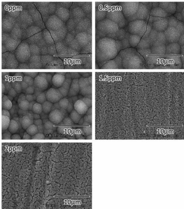
**Figure 17.** SEM images of the Ti specimen surface after the NaOH and heat treatments as a function of the Ca concentration in the NaOH solution. Apatite growth occurs between 0 and 1 ppm, with 1.5 ppm and above showing no apatite nucleation. Reprinted from Kizuki et al. [210] with permission from Springer Nature.
