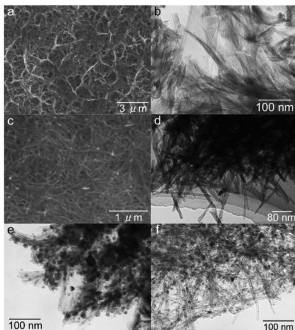
**Figure 22.** SEM (A,C) and TEM (B,D–F) images of NaOH-treated Ti plate (A,B), Calcined and NaOH-treated Ti plate (C,D), and silver acetate-treated of the NaOH-treated (E) and Calcined (F) samples, respectively. Exact sample methodology detailed by, and figure reprinted from Inoue et al. [252] with permission from John Wiley and Sons.
